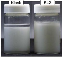
Rheopearl KL2 works as emulsion stabilizer to w/o system, especially to w/s system. Mechanism: Prevents water-phase particle from fusing and separating by increasing viscosity of outer phase (oil-phase).
