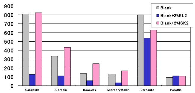
Rheopearl ISK2 could modify the hardness of anhydrous systems containing wax. On the other hand, Rheopearl KL2 softens anhydrous systems containing wax (such as lipstick) by inhibiting the growth of wax crystals.
