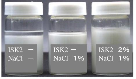
Rheopearl ISK2 enables water-and-silicone-only emulsions to be stabilized without solubilizers (such as ester oils), since ISK2 can be dissolved directly into the cyclomethicone portion of the silicone phase.
